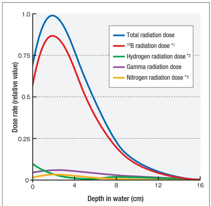
Figure 5. Depth Dose Distribution by Radiation Type
