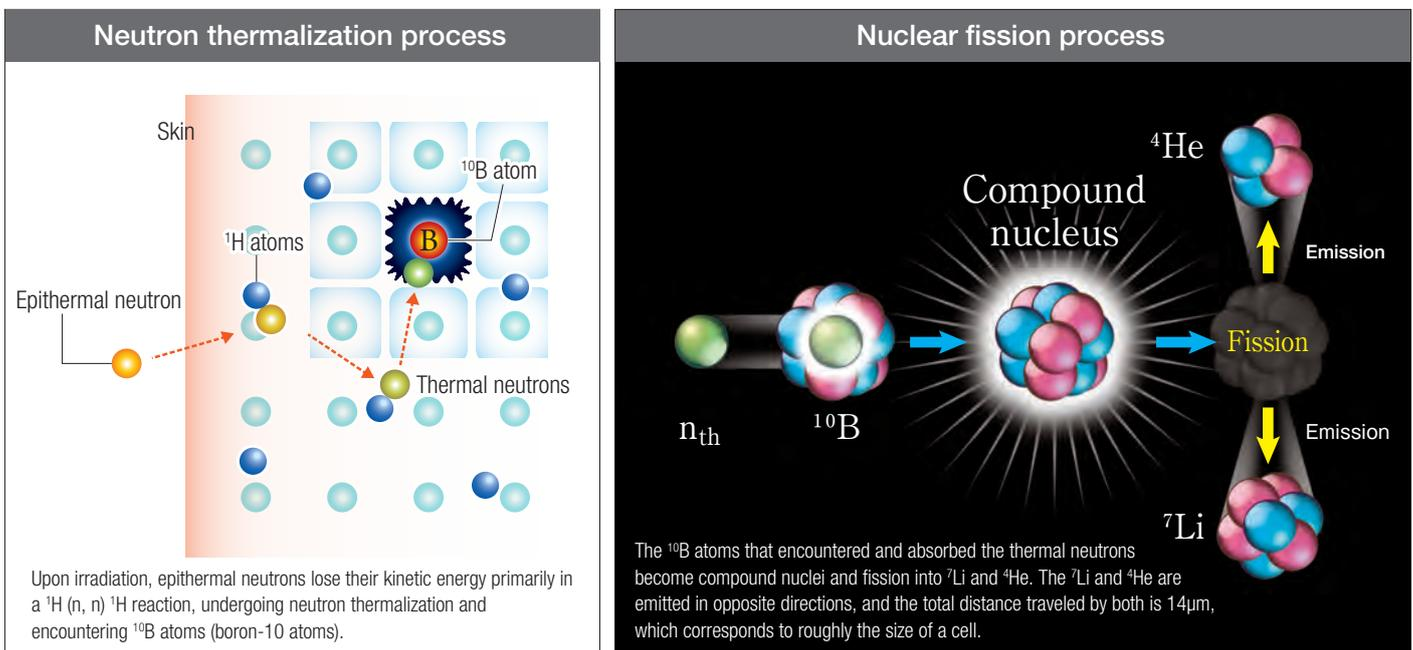
Figure 2. Epithermal Neutron Scattering Process and  $^{10}\text{B}$  Nuclear Fission Process
