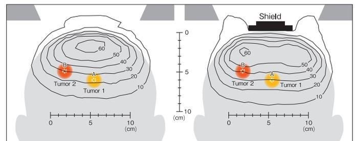
It is clear that by shielding the central part of the neutron irradiation field, it is possible to improve the relative depth distribution of neutrons (compare the doses at points A and B with and without the center shield).
