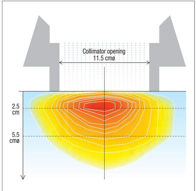
Figure 4. Two-dimensional Thermal Neutron Distribution
