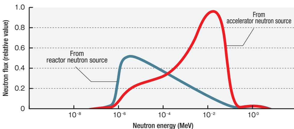
Figure 3. Epithermal Neutron Energy Distribution
