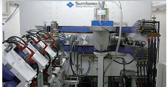
Photograph 2. Accelerator Neutron Source
